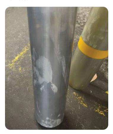
The Hubbard-Hall team discussed alternative fixturing of the parts and tried several different ways before determining that the original fixturing method was best for this application. Holloway and Valenti had them put the load back in, but this time directed the operator to put it all the way down. This proved to show a dramatic improvement in removing the lube, but a staining pattern was already present where the excessive lube contacted the tube.
