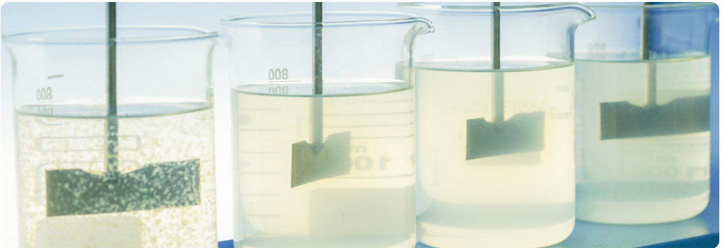
bench-testing, options for dosing both the clays and the liquid coagulant and flocculant.
