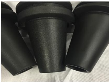
Manganese Phosphate over Machined Steel Parts. The middle part was Pickled with HCL; parts on the outsides were pickled with Acid Salt. Note the grainy appearance of the middle part.
