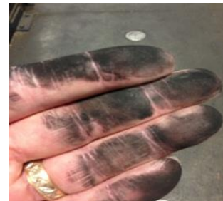
RIGHT: Over Pickling in HCL can result in carbon smut on the surface of parts.
