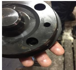
CENTER: Black Oxide over Machined Steel showing smear streaks.
