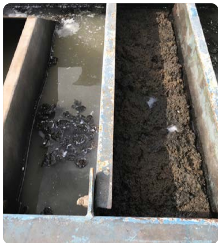
Before and after: SMP wastewater as seen prior to and after treatment with Hubbard-Hall’s AquaPure. Hubbard-Hall was able to help SMP reduce chrome to below 1ppm and make copper levels undetectable.
