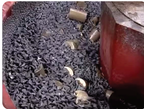
Aluminum billets tumbled with media and Lusterlume ALB-4
