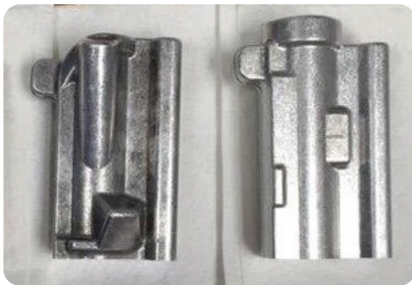
Finished aluminum rifle receivers: Left: Before vibratory cleaning process Right: Superior results after vibratory cleaning with Lusterlume ALB-4
