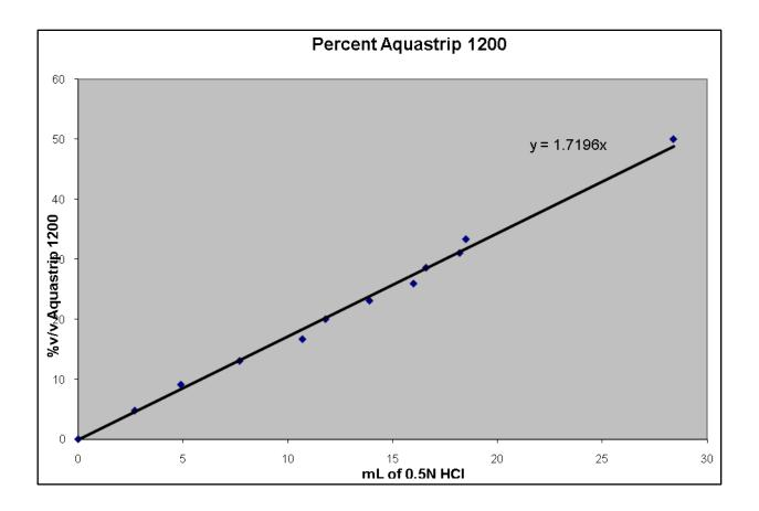
Note: If the color is too dark to accurately determine a Phenolphthalein endpoint, use a pH meter for the titration procedure. Titrate to a pH of 8.0
