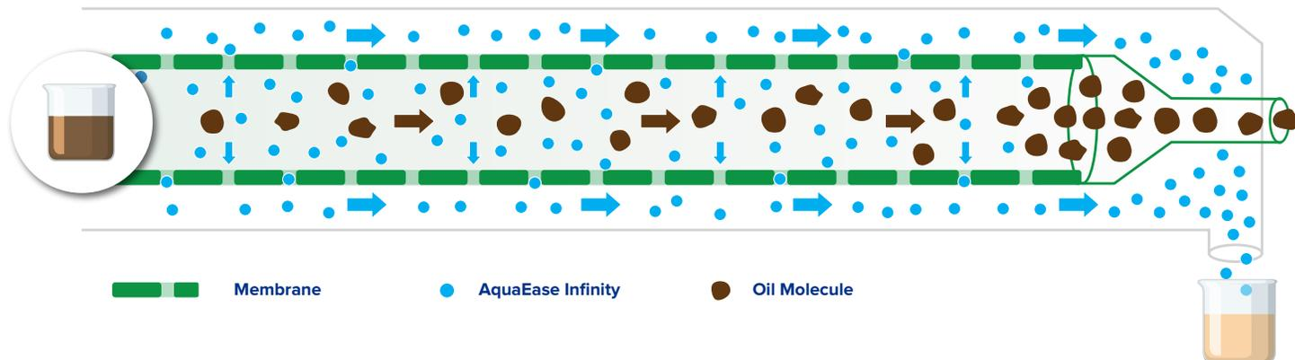
Most cleaners are not designed or suitable for membrane technology. AquaEase Infinity® cleaners are specifically designed for our membrane technology. The membrane separates the cleaner from the oil and soil, allowing the cleaning components to pass through its pores while trapping the contaminants inside. The reclaimed full-strength AquaEase® Infinity cleaner returns to the cleaning bath, fresh as new.
