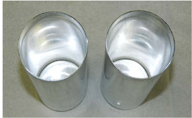
Aluminum extrusions after wash in Hubbard-Hall Emerald Acid Clean #1 at 9.13% for 6 minutes with a 2-minute factory water rinse and a 5-minute heated dry.
