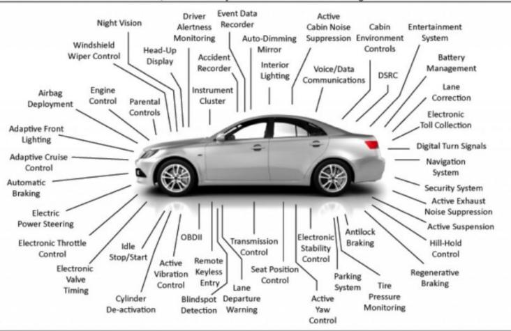
Current electronics on passenger automobile
