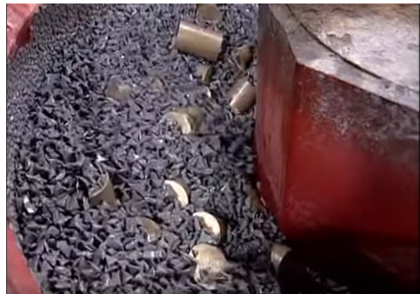
Aluminum billets tumbled with media and Lusterlume ALB-4
