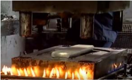
Forging Press provides extreme pressure to shape the desired part
