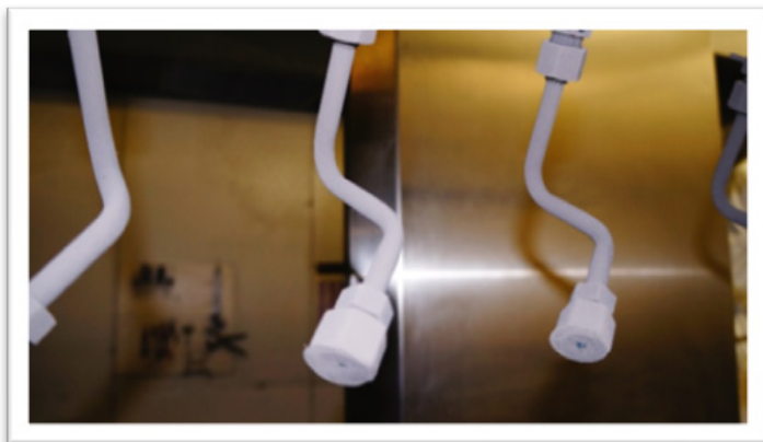
No need to throw away used flanges, covered in coating. Simply remove and strip for reuse.
