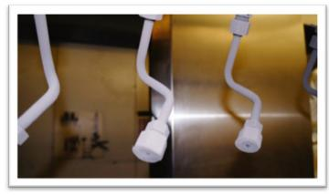
No need to throw away used flanges, covered in coating. Simply remove and strip for reuse.
