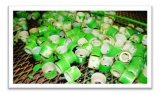
Reuse masking plugs up to 6-7 times before throwing away.
