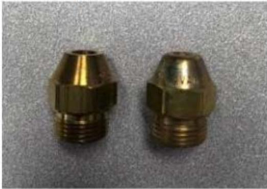
Image 1: Brass nozzle before on left. Nozzle on right is a reject due to pitting from the Nitric brite dip process
