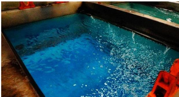
*Figure 2 Clean rinse water is critical in the barrel cleaning line*
