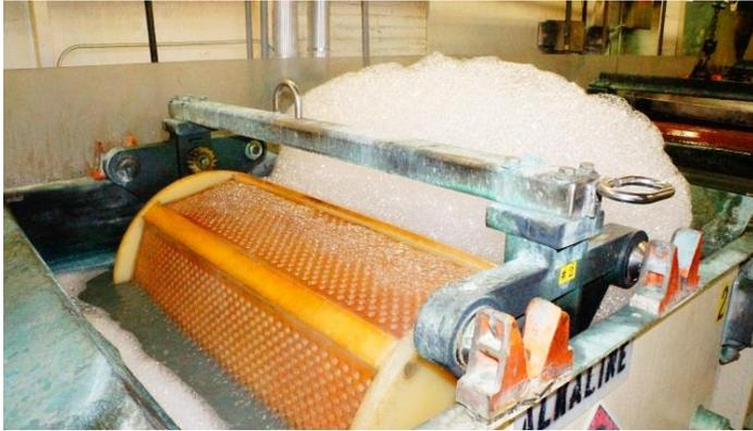
*Figure 4 the proper amount of foam in the Aquaease SL 80 is important for complete cleaning in this barrel tumbling line*
