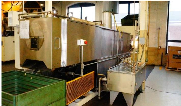
*Figure 5 The spiral washer provides consistent reliable cleaning with Aquaease PL 72 A32*
