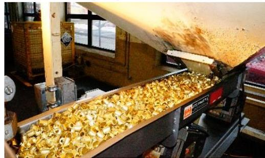
*Figure 1: Brass ferrules being fed into the Jenfab spiral washer*
