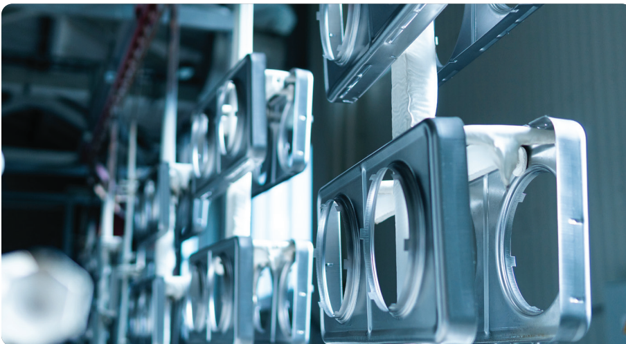
Mi-Phos 22PW EX cleans steel, zinc plate, aluminum, and terne plate while adding a tenacious phosphate undercoating all in a single step.
