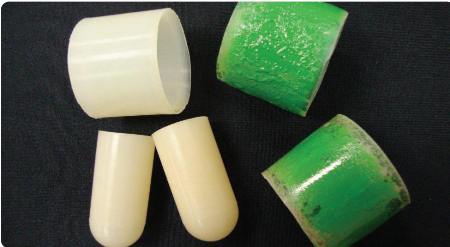
Placed on tubes prior to powder coating, masking plugs cleaned with Aquastrip ACB, can be reused 6-7 times before being thrown away.
